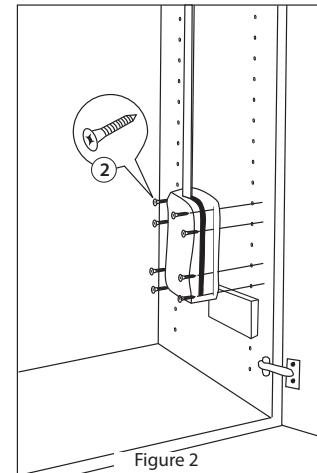
3. Using the wooden guide for height, place the right side mechanism into position and insert a minimum of 8 screws (2), for best results use 12 screws (2) (See figure 2).
