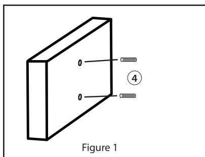
1. Insert the wooden dowels into the wooden positioner back (See figure 1).
